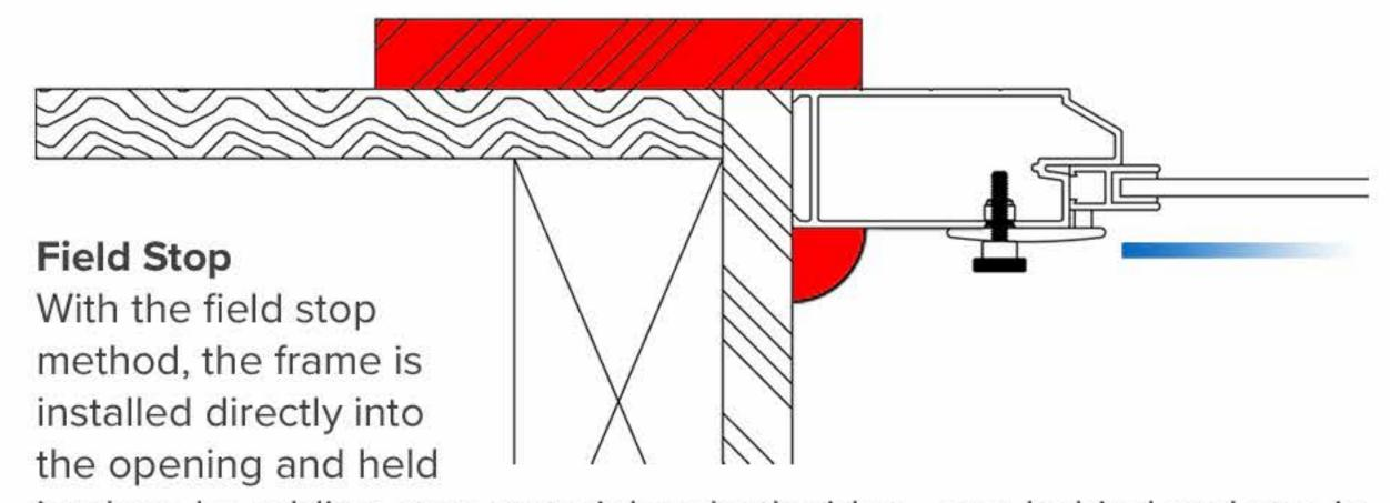
in place by adding stop material on both sides—one behind and one in front—pinning the frame securely in place. This can be done using the structure itself or additional materials of choice. With this option, Casco will undersize the frame dimensions by 1/2" to allow for proper fit within the channel.
