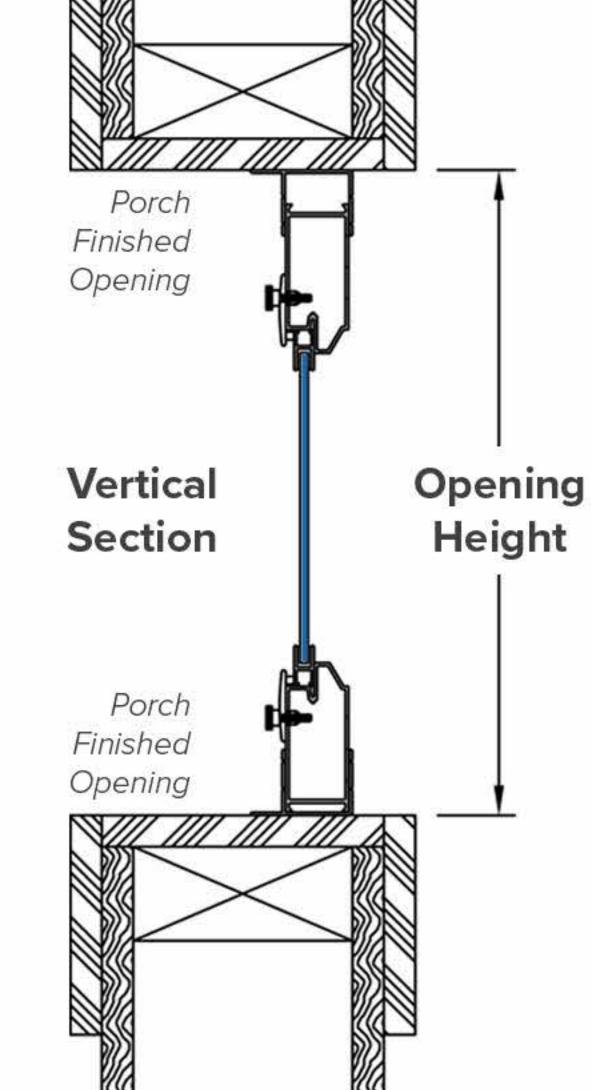
Note: The system was designed for porches, patios, and other outdoor living spaces. While glass panels are available, it is not intended to function as a fully sealed window system. As with screen porches, some water infiltration may occur. Ensure the finished opening allows for proper drainage to the exterior.
