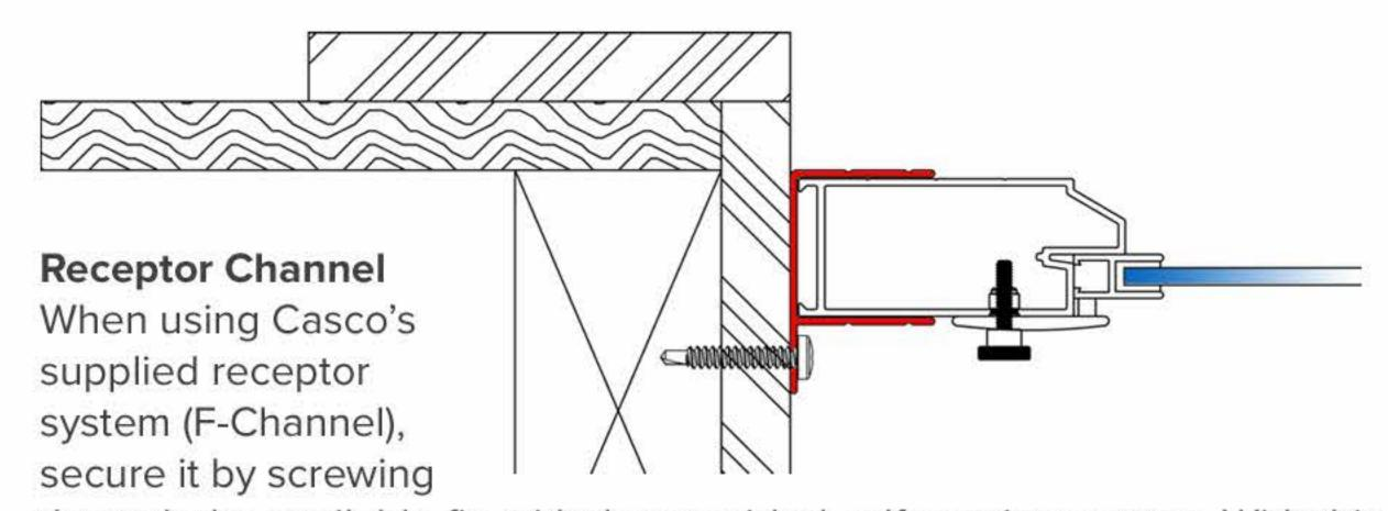
through the available fin with the provided self-tapping screws. With this installation method, Casco will undersize the frame dimensions by 1/2" to allow for proper fit within the channel.
